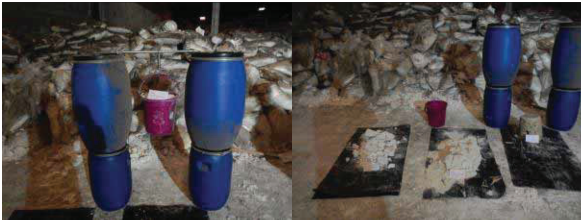
Figure A1.27 Determination of specific weight of POP pesticides (left) Specific weight POP pesticides, right most set is wet pesticides (right)
