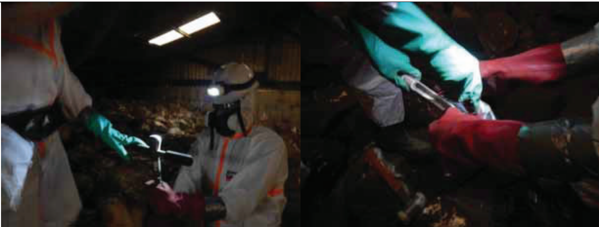
Figure A1.9 Manual drilling through wastes (left) Transfer of samples to sampling bags (right)
