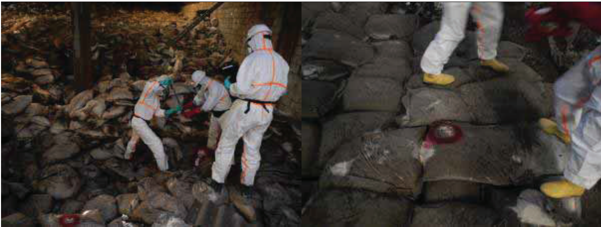
Figure A1.8 Sampling of wastes in warehouse 5 (left) Spray painting the sampling location (right)
