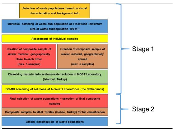
Figure 5.1 Sampling procedure POP-pesticides bags in two stages
