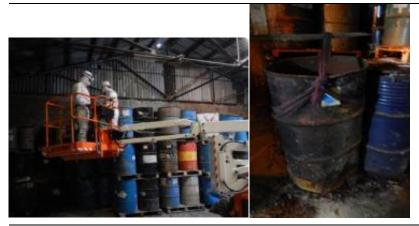
Figure 5.3 Banding of drums (left). Individual weighing and transport of drums (right)
