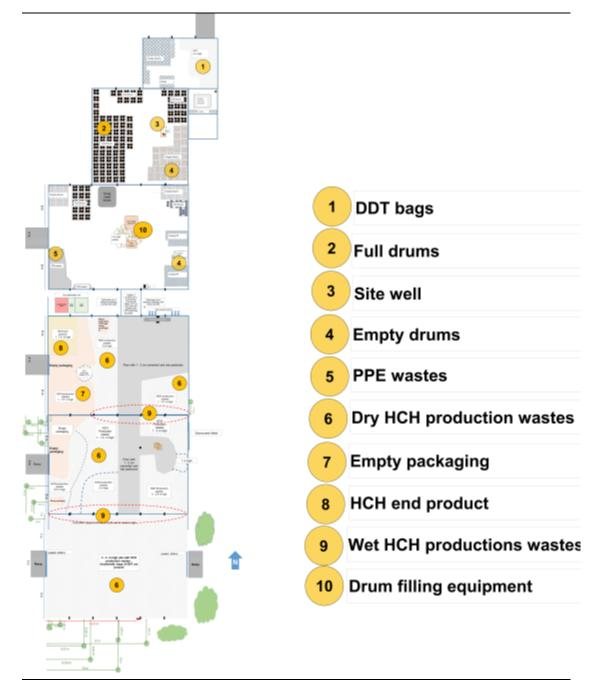
Figure 9.1 The site location sketch illustrating the Conceptual Site Model of the warehouse
