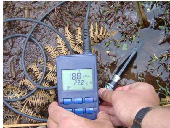
Groundwater seep (with very low electrical conductivity!!) South-Pare mountains, Tanzania
