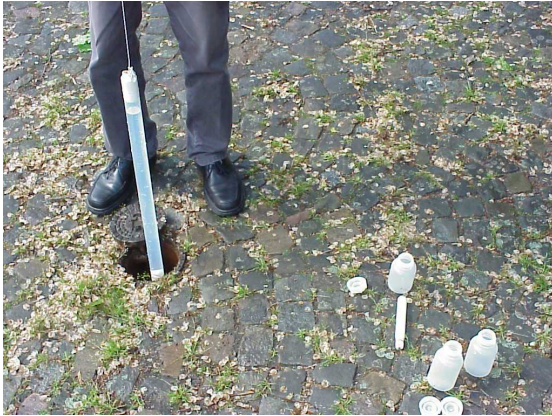
Sampling a 60 m deep groundwater well in Limburg, The Netherlands
